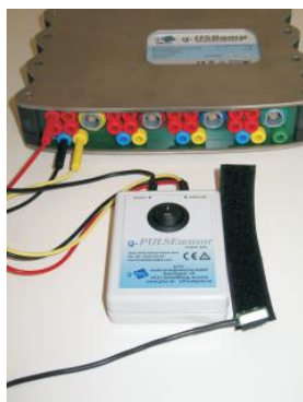
Figure 3: Pulse rate sensor with biosignal amplifier
