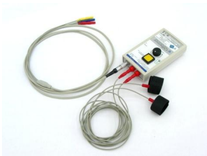
Figure 7: Galvanic skin response sensor for finger mounting (finger electrodes)
